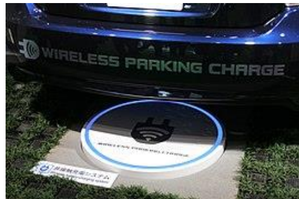
Detail of the wireless inductive charging device
