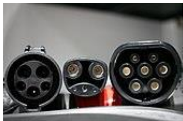
IEC Type 1/SAE J1772 inlet (left); NACS (center); IEC Type 2 connector outlet (right) Common connectors include Type 1 (Yazaki), Type 2 (Mennekes) , Type 3 (Scame) , CCS Combo 1 and 2, CHAdEMO and Tesla. (25)(26)
