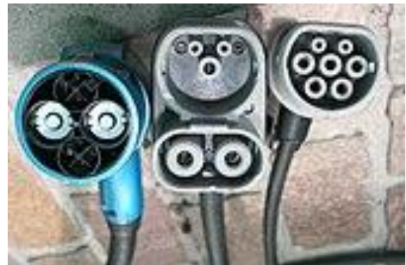
IEC Type 4/CHAdEMO (left); CCS Combo 2 (center); IEC Type 2 outlet (right)
